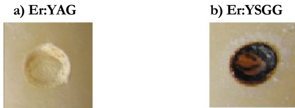
Fig. 9: Pictures of cavities in dentin, made with Er:YAG and Er,Cr:YSGG lasers following three consecutive laser pulses of the same laser pulse fluence of 80 \text{ J/cm}^2 [19]. In order to eliminate any influence of the difference in pulse duration, the Er:YAG pulse duration (Fotona dental laser, VSP mode) was adjusted to match that of the Er,Cr:YSGG (Waterlase PFN S mode). In this experiment, no water spray was used.
