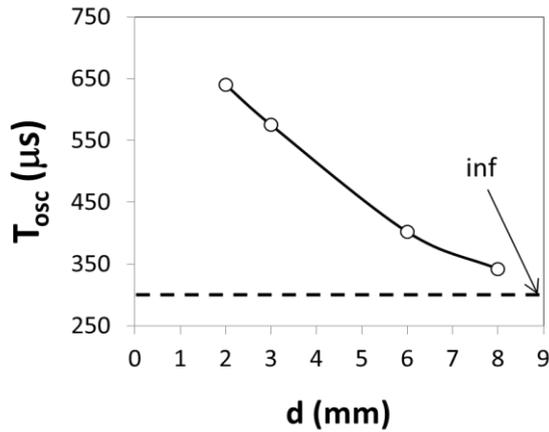
Fig. 2: Measured dependence of the bubble oscillation period  $T_{osc}$  on the diameter of the canal, for laser pulse energy of 20 mJ. The dotted line represents  $T_{osc}$  in an infinite reservoir.
