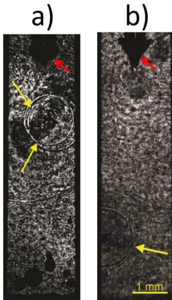
Fig. 5: a) Primary shock wave emission following the SWEEPS-accelerated collapse of the initial bubble; b) Secondary shock waves are also emitted along the wall canals as a result of the collapse of secondary bubbles, which are generated deeper in the canal during the initial bubble's growth and collapse. Yellow (long) arrows point to the emitted shock waves and red (short) arrows show the growing bubble of the subsequent laser pulse.
