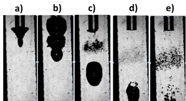
Fig. 9: Sequence of images showing the development of cavitation bubbles during an Auto SWEEPS cycle for the laser pulse separation of  $T_p < T_{opt}$ . A subsequent bubble forming very quickly following the initial bubble is shown in Figs a) and b). The bubble’s “propulsion” deeper into the canal can be seen in Figs c) and d).
