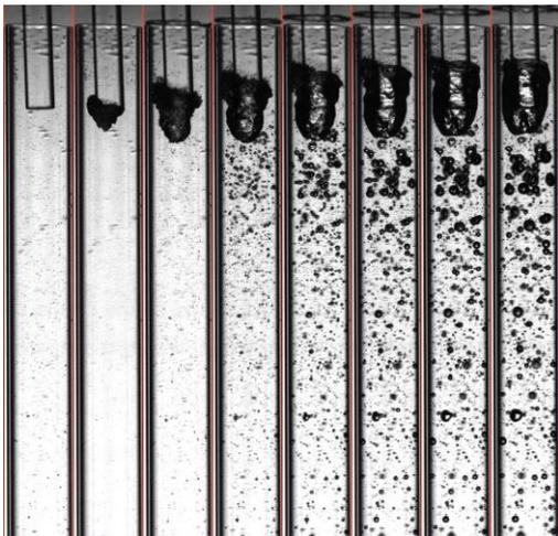
Fig. 3: High-speed camera temporal sequence of images of the development of an initial bubble close to the fiber tip, accompanied by smaller secondary bubbles forming throughout the blind canal, as observed following the emission of a single laser pulse. Time increment between images is 40  $\mu s$ .
