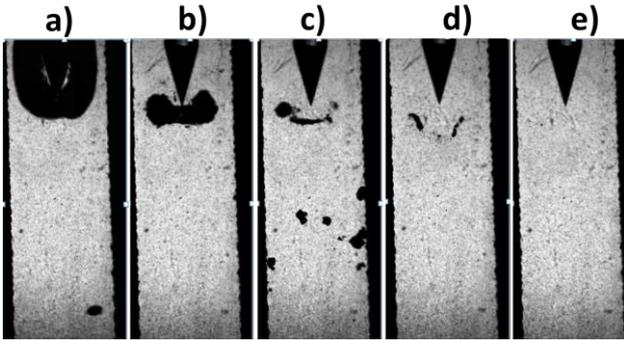
Fig. 10: Sequence of images showing the development of a cavitation bubble following a single PIPS Er:YAG laser pulse. The bubble cavitation is located predominantly close to the conical PIPS fiber tip.
